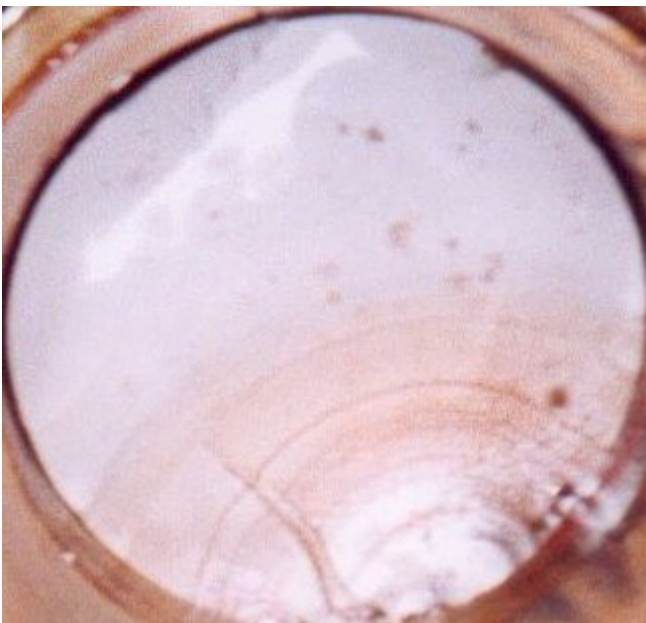
Visible beachmarks on a tiebolt failure
