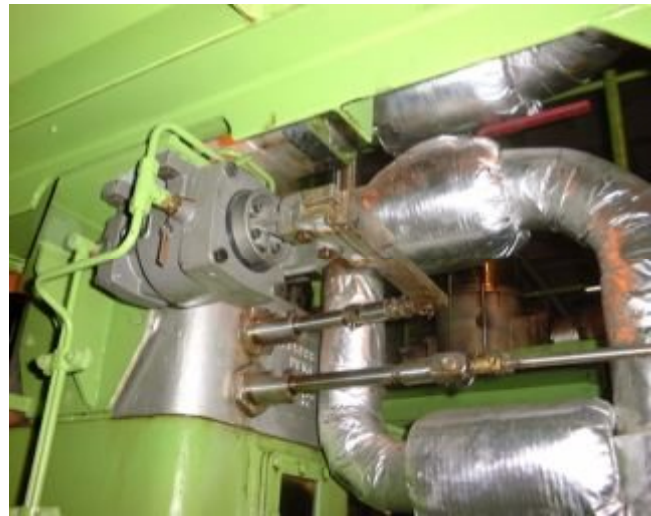
Fuel Quantity and VIT Linkages on Engine
