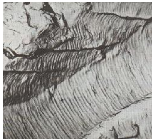
Magnification of fatigue failure showing striations
