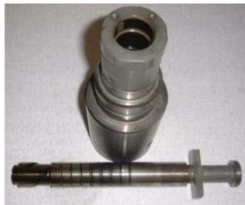
Plunger and barrel from a Sulzer ZA40
