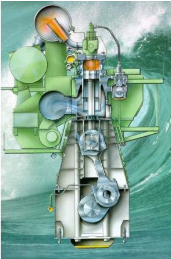
MAN B&W MC series uniflow scavenged engine
