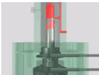
Quantity Control Using Fuel Rack
