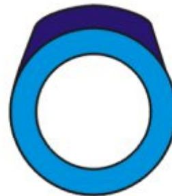
Inlet or exhaust valve cam for unidirectional medium speed engine. The cam has to open and close the valve smartly without shock loading
