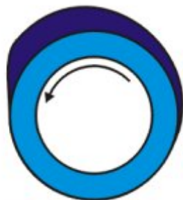
Fuel Cam for unidirectional medium speed engine. The cam has fast lift for injection and a slow return to avoid shock loading
