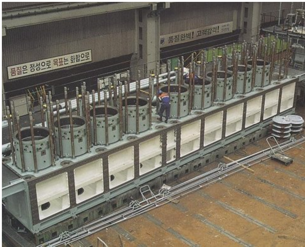
Entablature Mounted On A Frame With Liners In Place
